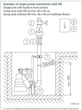
In case of installation beneath the backpressure level the pressure tube must be taken in a loop over the local backup level acc. to EN 12056. Besides, it must be secured with an EN 12050-4-proofed swing-type check valve. Additionally we recommend an alarm system.
